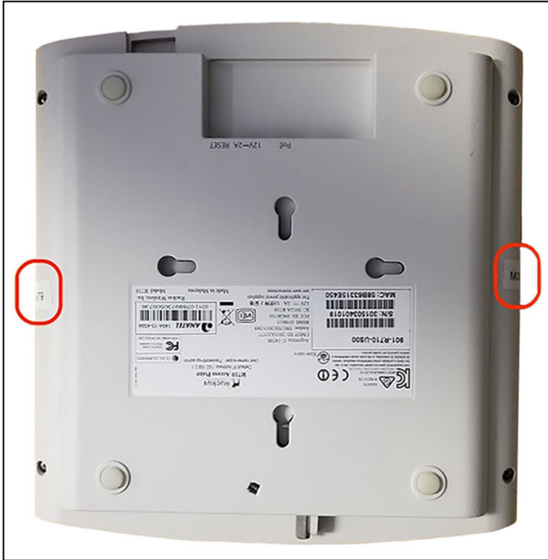
FIGURE 155 R710 AP Seals (Bottom View)
