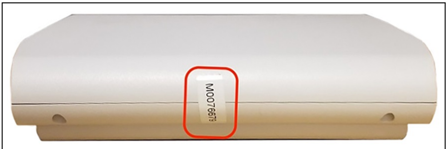
FIGURE 153 R710 AP Side Seal
