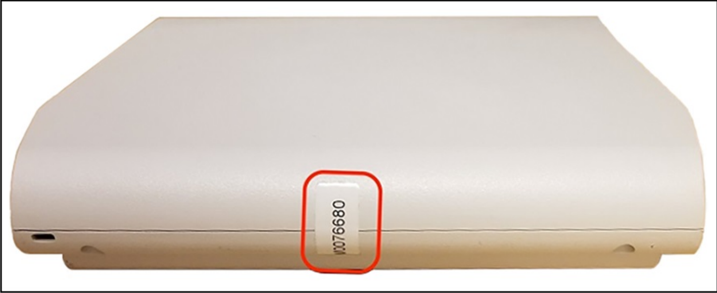
FIGURE 154 R710 AP Side Seal (Opposite Side)
