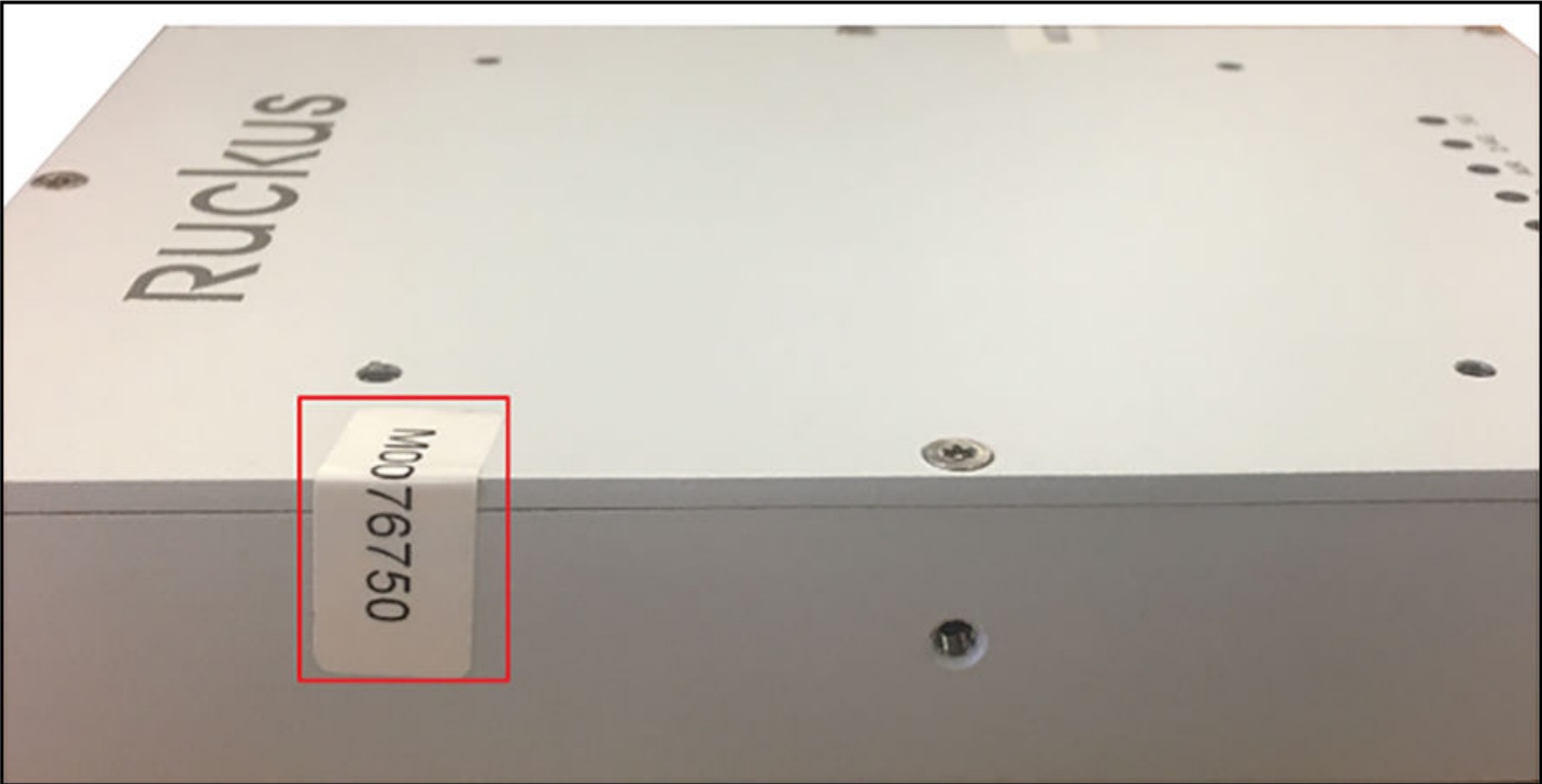
FIGURE 160 E510 AP Seal (Top-Left View)
