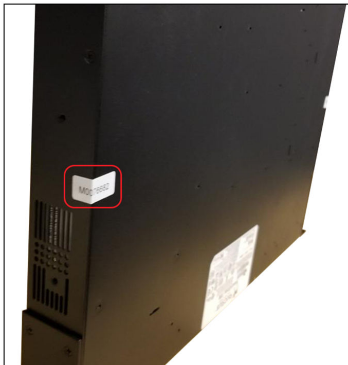
FIGURE 140 SmartZone 100 Side Seal (Vertical View)
