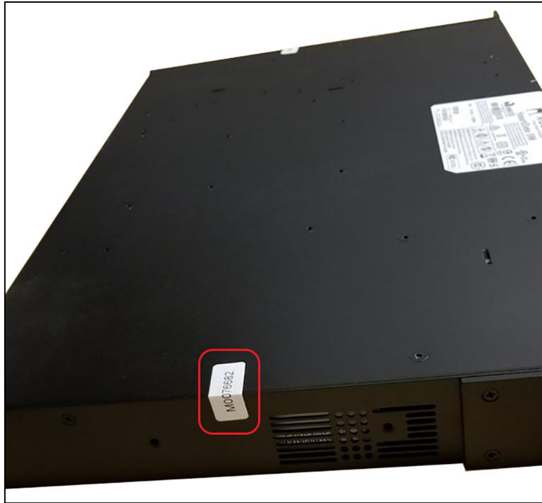
FIGURE 140 SmartZone 100 Side Seal (Vertical View)
