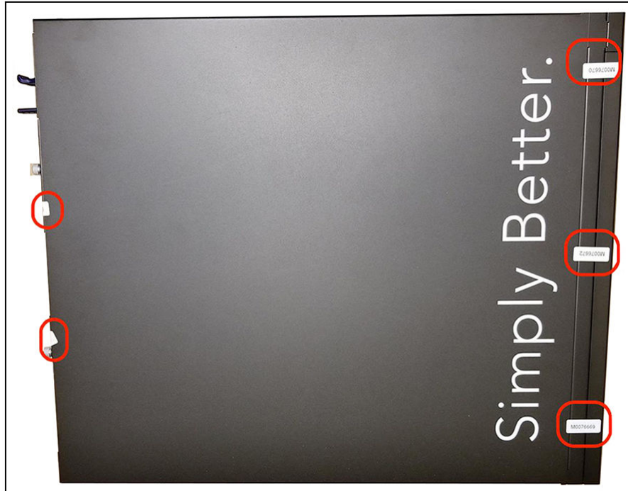
FIGURE 144 SmartZone 300 Rear Seals
