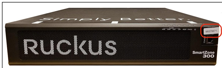
FIGURE 145 SmartZone 300 Front Seals
